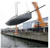
VARUNA is an extremely lightweight yacht, sophisticated down to the last detail. Characteristic features are the long bowsprit, the machined stainless steel keel fin and the narrow rudder.
